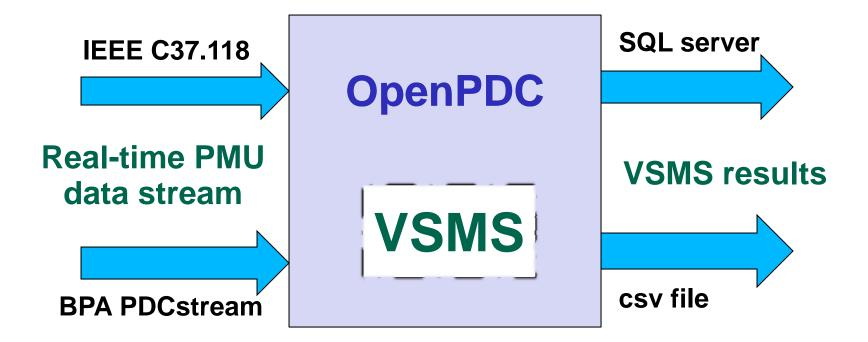
VSMS action adapter built into OpenPDC early release. Being moved to 64 bit version 1.4 sp1. Available for beta testing in October 2011.
