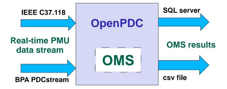
OMS action adapter built into OpenPDC 64 bit version 1.4 sp1. Available for beta testing.
