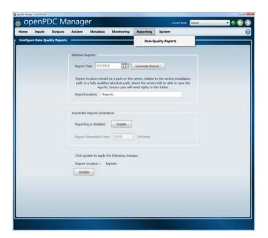
New with the latest build (Version 2.0.118 or later) of the openPDC is the ability to automatically produce the daily report shown above to get a quick summary of the status of devices connected to the openPDC. Implemented as a generic class in the Grid Solutions Framework this new capability is extensible for routine reporting on other performance metrics within the performance historian.
